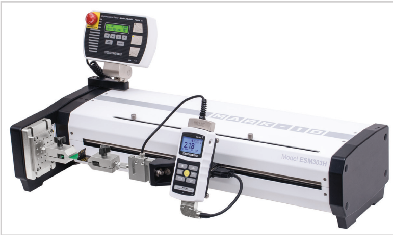
^ ESM303H is shown above configured for a peel test, with a Model M71 indicator, Series R01 load cell, and G1008 film and paper grips.
