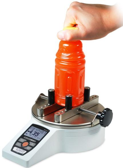
Thank you for purchasing a Mark-10 Series TT01 digital cap torque tester, designed to measure bottle cap application and removal torque.
