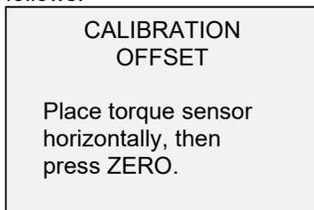
5. Place the tester on a level surface free from vibration, then press **ZERO**. The tester will calculate internal offsets, and the display appears as follows:
