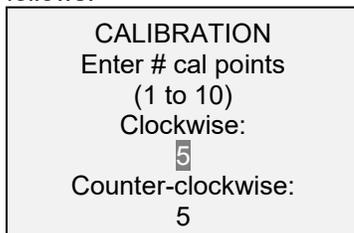
The tester can be calibrated at up to 10 points in each direction. Enter the number of calibration points for each direction (clockwise and counter-clockwise). At least one point must be selected for each direction.
