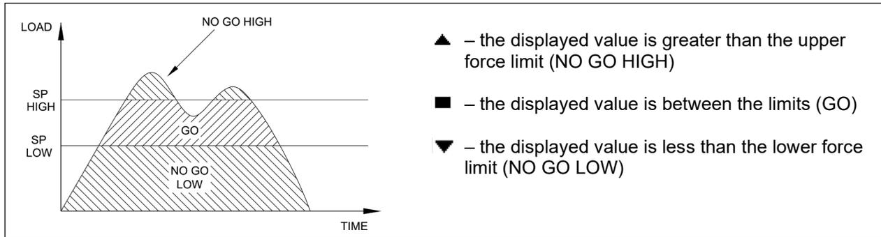
**Note:** Set point indicators reference the displayed reading, not necessarily the current live load.
