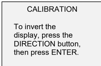
2. Press **DIRECTION** to invert the display, if desired. **ENTER** to continue. The display appears as follows:
