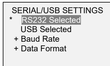
Select either RS-232 or USB input (output is always simultaneous through both the USB and RS-232 ports). Communication settings are permanently set to the following:
