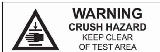
**Definition:** Keep any body parts and clothing clear of the area between the base of the test stand and the moving crosshead.
