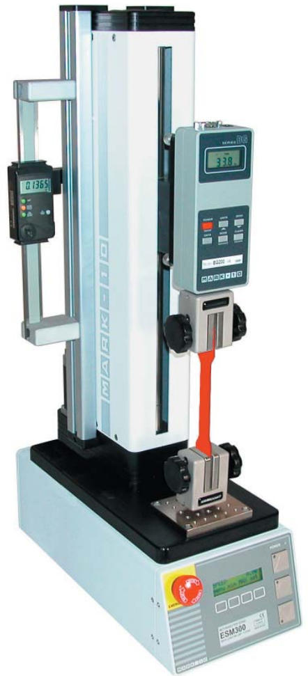
The ESM300 is shown in a typical tensile testing application, with Series BG digital force gauge, digital travel display, and parallel jaw grips
