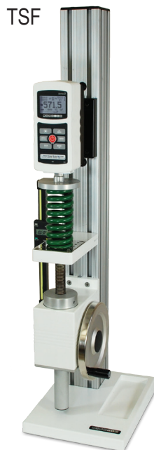
The TSF is shown testing a compression spring, with a Series 5 digital force gauge and digital travel display
