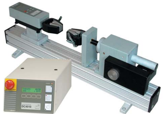
The TSFM500H-DC is shown set up for a tensile test, with Series CG digital force gauge and wedge grips.
