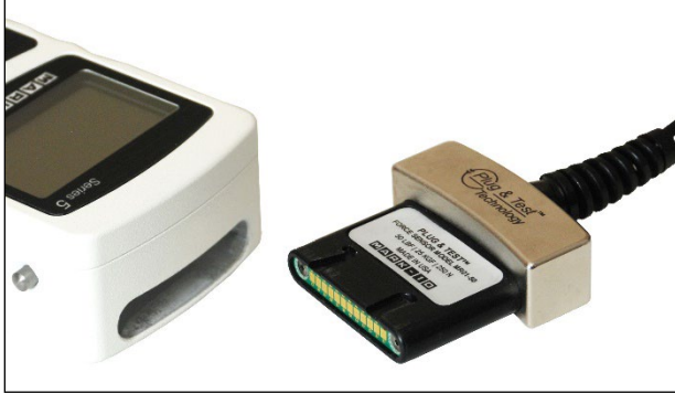
Fig. 3.1 Appropriate orientation of the Plug & Test® connector.
