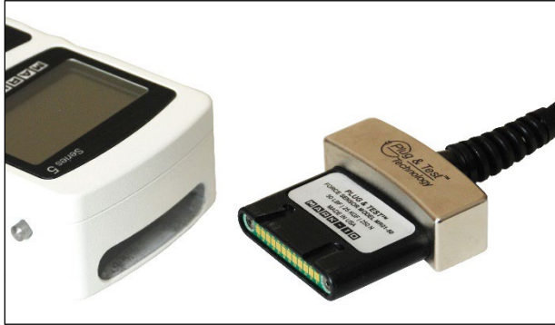
Fig. 3.1 Appropriate orientation of the Plug & Test® connector.
