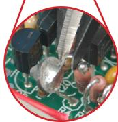
Using a pair of wire cutters, cut the connection between the components.
