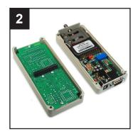
The separated halves appear as above. The PCB of interest is the auxiliary PCB, shown on the right half, adjacent to the battery. Remove the battery before beginning work on the modifications.
