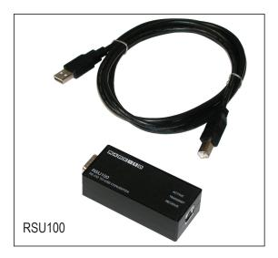
**Model RSU100:** Converts RS-232 signals into USB, typically used for transmitting data from a Mark-10 test stand control panel to data collection software on a PC. A USB cable is included.
