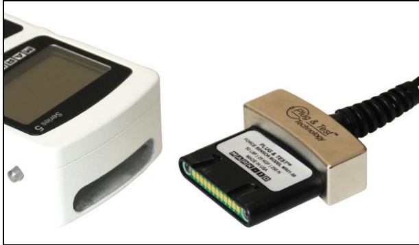
Fig. 3.1 Appropriate orientation of the Plug & Test® connector.
