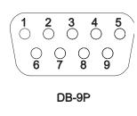
1. RS-232 receive RS-232 transmit 3. Mitutoyo request External trigger Input bit 3 4. Mitutoyo clock "Within" set point output Output bit 2 5. Signal ground 6. N/A 7. +9-12V DC Mitutoyo ready
