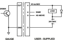
volatile memory of the insMtrument and all readings are compared to these limits. The results of the comparisons are indicated through the three open-collector outputs provided on the 9-pin connector, thus providing "under", "in range" and "over" signaling. These outputs can be connected to indicators, buzzers or relays as required for the application. Refer to Section 8 for command details.
