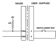
signal is applied. It is possible to capture the reading with a normally open contact (high to low transition of the trigger signal) or a normally closed contact (low to high transition). In "edge" mode, the RG will output the captured reading and hold this reading until the command CLR is sent prior to a new test. The "level" mode provides for the display to hold the reading only until the trigger signal returns to its original state. Refer to Section 8 for command details.
