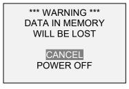
If no option is selected, this screen will be displayed indefinitely, or until battery power has been depleted.
