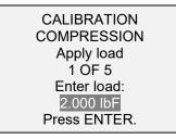
Use the **UP** and **DOWN** keys to adjust the load value as required. The load values default to even increments, as indicated by the previously entered number of data points (even increments are recommended for best results). For example, if a 50 lbF capacity gauge is calibrated, and 5 data points were selected, the load values will default to 10, 20, 30, 40, and 50 lb. Apply the calibration load. Then press **ENTER**.
