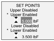
One, two, or none of the set points may be enabled. To toggle between the tension and compression directions, press the **DIRECTION** key.
