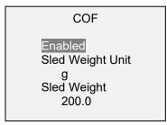
Available sled weight settings: 10% to 100% of the gauge capacity
