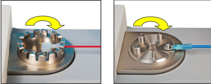
2. Insert the loose end of the wire between the cams in the mechanism. Keep the wire taut as it is inserted. If auto-start is enabled, the test will begin when the switch is activated (refer to later sections for operational details). Refer to the image below:
