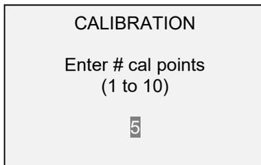
The tester can be calibrated at up to 10 points. Enter the number of calibration points (at least one point must be selected).
