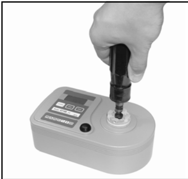
Fig. 1 Gradually exert torque to achieve accurate results
